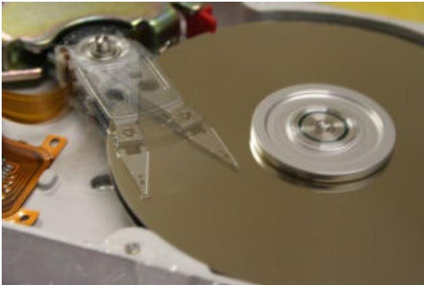
Internal view of a hard drive in operation. The arm appears blurred due to its rapid movement.
